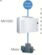
The simple configuration for running standard high voltage motors directly realizes highly effcient operation with minimal loss due to input/output voltage transformers.
