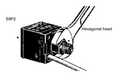
When attaching the Mounting Bracket to the Sensor, make sure that each M3 screw is tightened to a torque of 0.5 N•m (0.37 ft•lbs) max.
