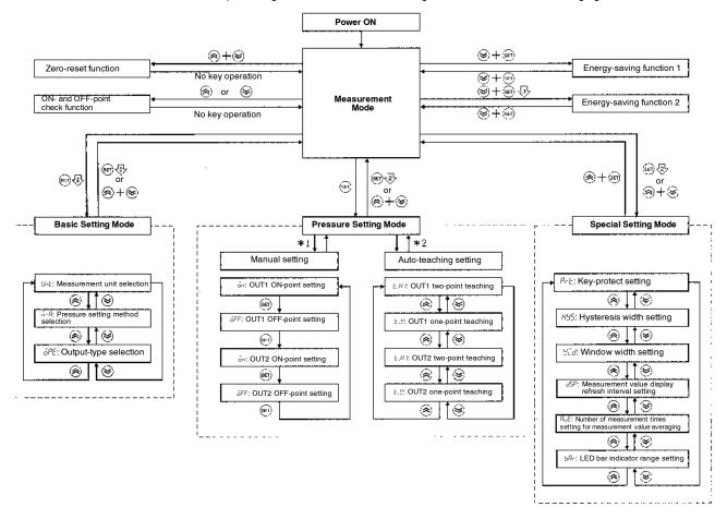
Note: 1. (a) and (b) indicate that the key must be pressed for approximately 2 or 3 s respectively.
