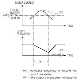
\*2. If the output current does not become set level or less, the operation will be held at the min. output frequency.
