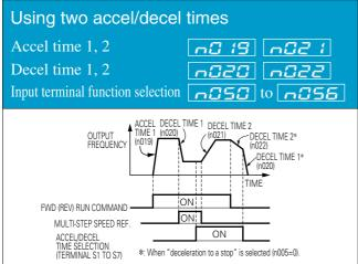
By setting input terminal function selection (one of n050 to n056) to "8" (accel/decel time select), accel/decel time is selected by turning ON/OFF the accel/decel time select (one terminal of S1 to S7).
