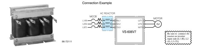
When power capacity is significantly greater when compared to inverter capacity, or when the power-factor needs to be improved, connect the AC or DC reactor. In order to suppress high harmonic wave, DC reactor can be used with AC reactor.
