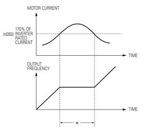
\*: Holds the acceleration to prevent the motor from stalling.
