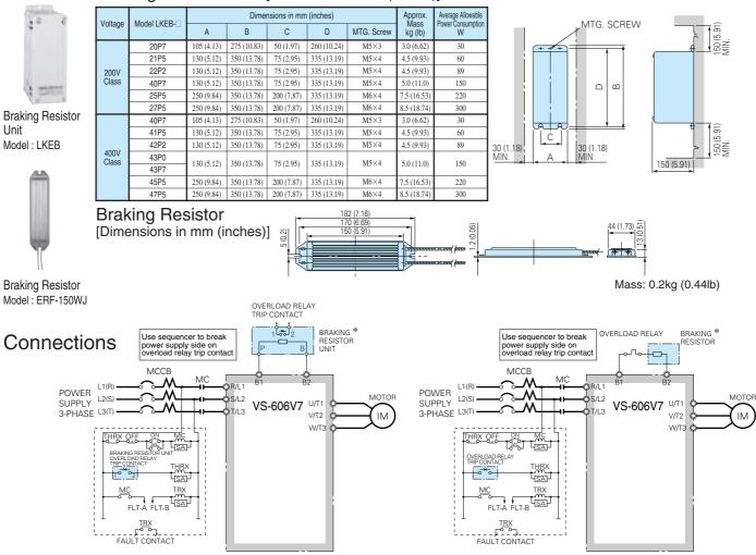
\* When using a braking resistor (option), set the stall prevention during deceleration to "Disabled" (n092=1) or the motor might not stop within the set deceleration time. Notes:
