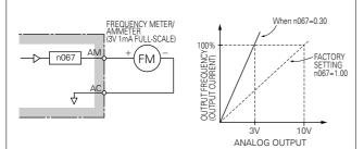
Set analog output voltage at 100% of output frequency (output current).
